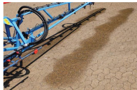
Designed to ensure even spray distribution on both sides of the boom when the nozzles are installed in alternating directions
